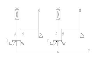
D = Air connection A = Outlet Flow Divider
